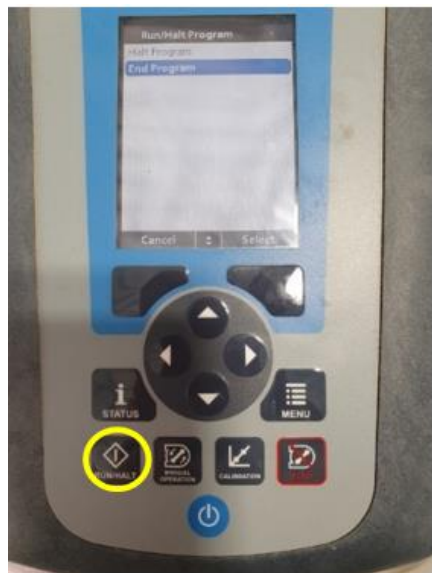
FIGURE 54 – PRESSING RUN | HALT BUTON IN AS950 CONTROLLER
