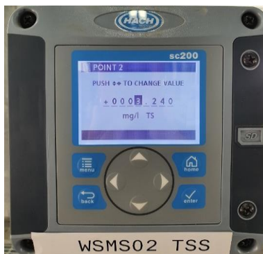
FIGURE 26 – ENTERING CALIBRATION POINT 2 (MID)
