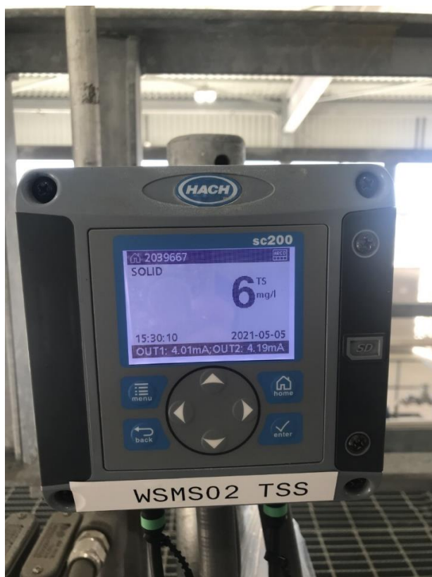
FIGURE 10– RECORD TSS READING FROM SC200 (ENSURE READING IS FROM THE ONLINE TSS PROBE)
