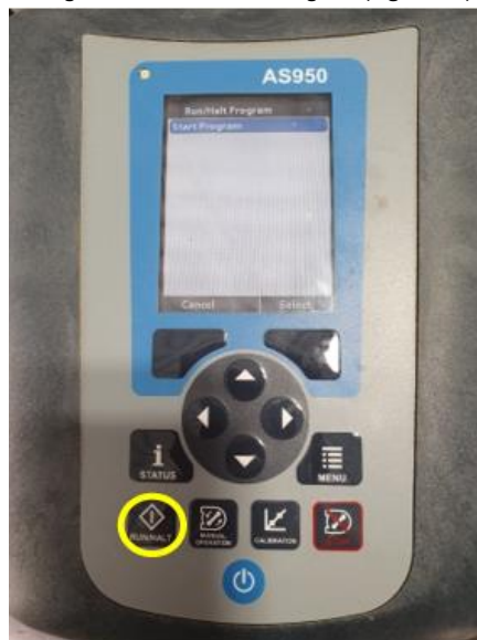
FIGURE 55 – PRESSING RUN | HALT BUTTON AGAIN AND START PROGRAM IN AS950 CONTROLLER
