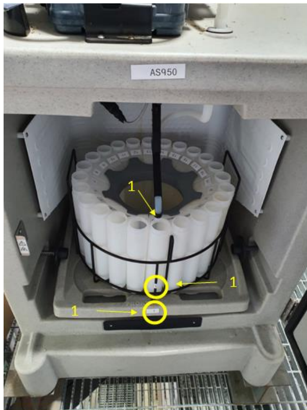
FIGURE 53 – REPLENISHING OF CLEAN VIALS IN AUTOSAMPLER ENSURING THAT BOTTLE 1 LINES UP WITH POSITION 1
