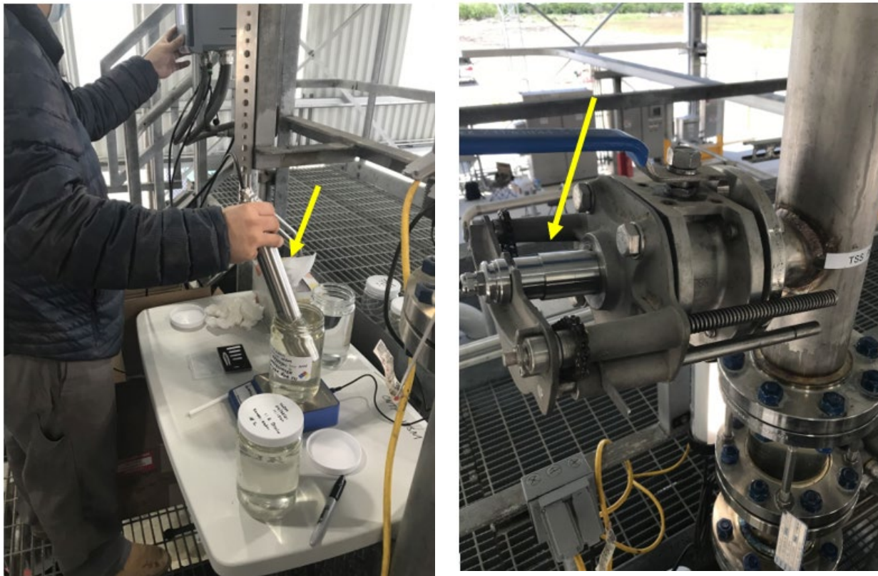
Photograph J TSS Automatic Sampling Device - During Calibration (Left) and Mounted (Right) April 23, 2021, and May 5, 2021, respectively
