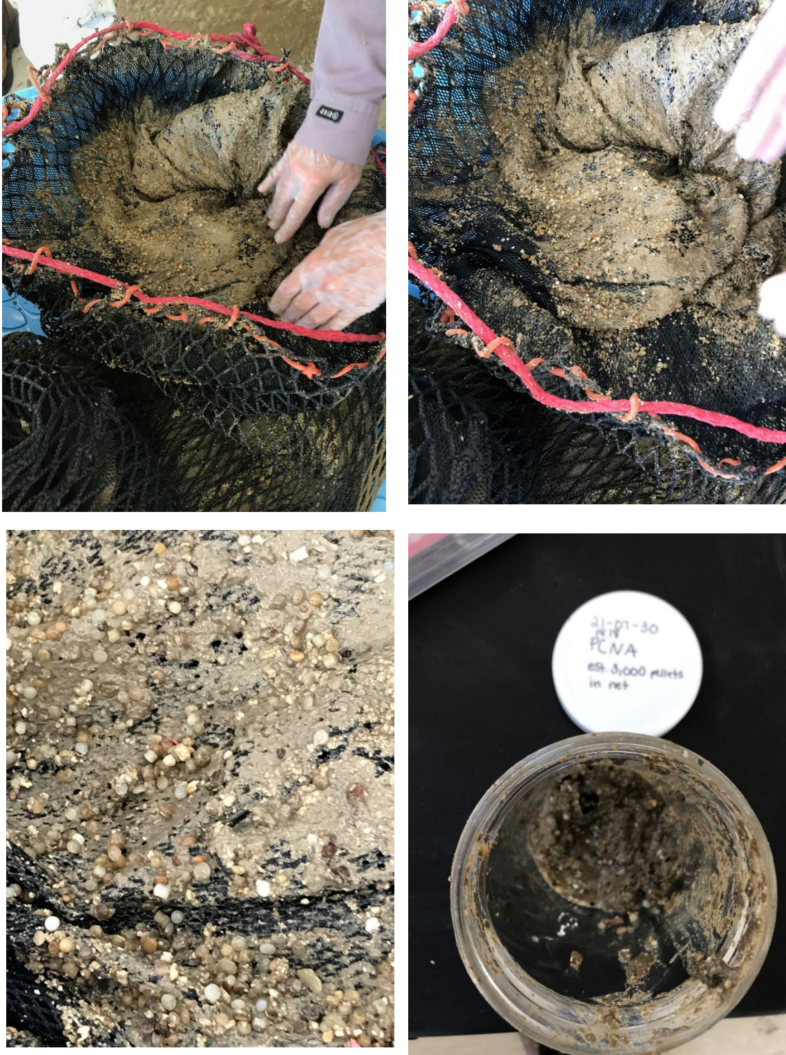
Photograph P Thousands of Pellets in Pellet Capture Net at WSM – In the Top Two and Left Bottom (Left) and Recovered in Jar (Right Bottom) July 30, 2021
